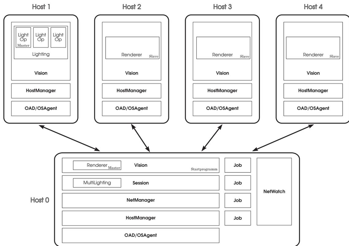
Figure 3: Example of a running distributed system. The NetWatch application currently monitors the activities of objects on host 0. Information about objects on other hosts can be accessed by instantiating their Observer interface with a Job object.
