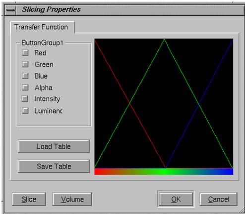
Figure 2: Scalar values can be mapped onto slicing planes by an interactively adjustable transfer function.
