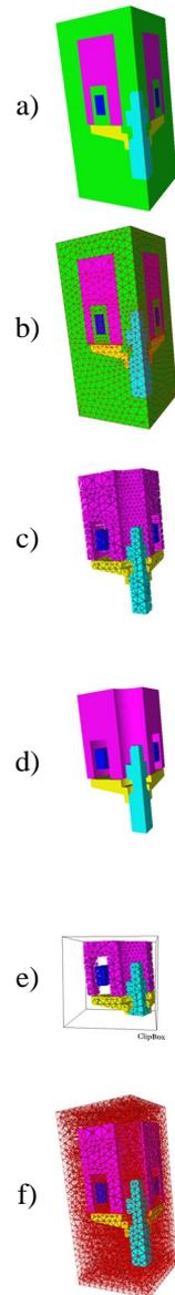
Figure 9: The rendering subsystem has several rendering modes for close examination of detail or interactive rendering of general shape. The images above show a partitioned dataset. Each partition can be turned on/off independently. Each mode or a combination of modes can be applied to each partition separately: a) surface b) surface and edges c) volume elements of adjustable size d) surface of partition e) element-oriented clipping f) volume element edges
