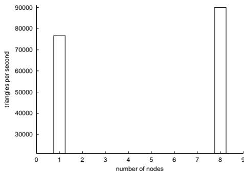
Figure 8: System saturation observed when using all 8 processors of 1 node (left) compared to 1 renderer on 8 nodes (right).
