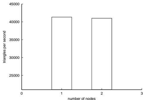
Figure 7: Comparison of assigning 4 renderers to 1 node (left) or 1 renderer to 4 nodes (right).
