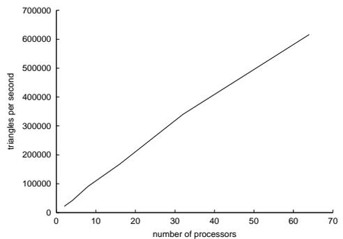
Figure 5: Scaling of the rendering subsystem in terms of number of processors used.
