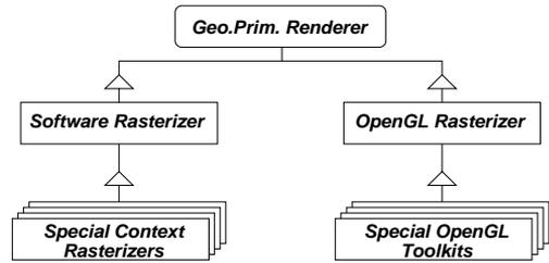
Figure 3: The rendering subsystem derives several software based rasterizers and hardware accelerated implementations from a single well defined interface.
