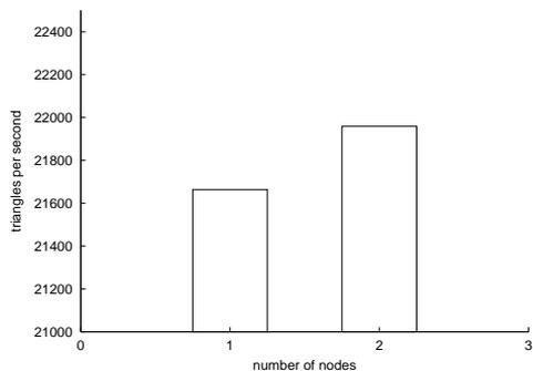
Figure 6: Comparison of assigning 2 renderers to 1 node (left) or 1 renderer to 2 nodes (right).
