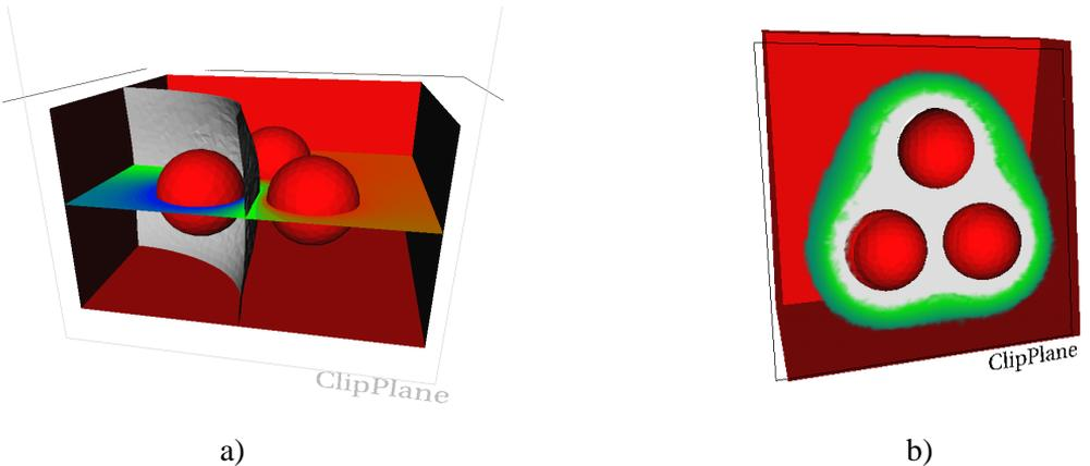
Figure 11: Two examples of possible direct visualization: On the left is an electrostatic simulation showing some special scalar value as an isosurface and a color-mapped slice through the unstructured simulation grid, on the right is the same dataset now with a simulation of heat dissipation. The three spheres are heated and the resulting scalar field is rendered directly from the unstructured grid using volume rendering.
