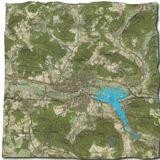
Figure 11: The carpet method on large complex terrain. Even though the particle system is sparse, the carpet provides a closed water surface (particle size exaggerated compared to real world scale). We use 8000 particles at 26 fps.
